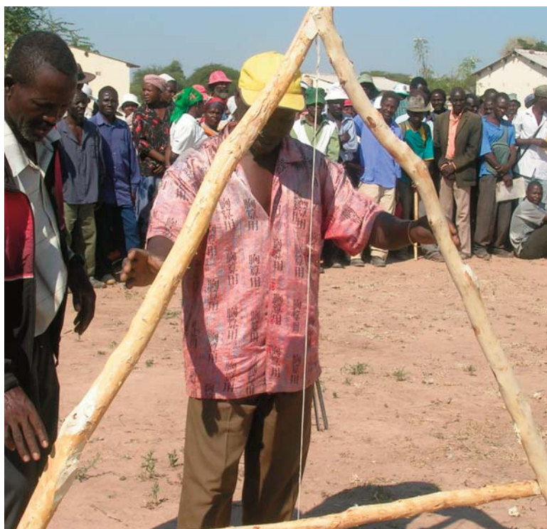
Community-driven training on soil and water management using a locally-made A Frame in Gwanda district, Matebeleland South Province, Zimbabwe Irvine Siyafa, 2007
